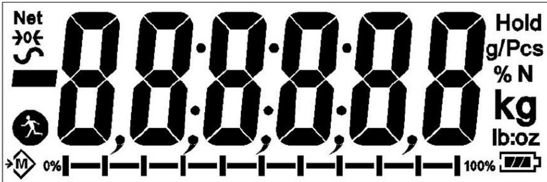
Other symbols will show when a weight has been tared (NET) the scale is at zero and stable, if a value has been stored in memory or when the animal weighing function has been enabled. A battery symbols will show the state of charge of the internal battery.
