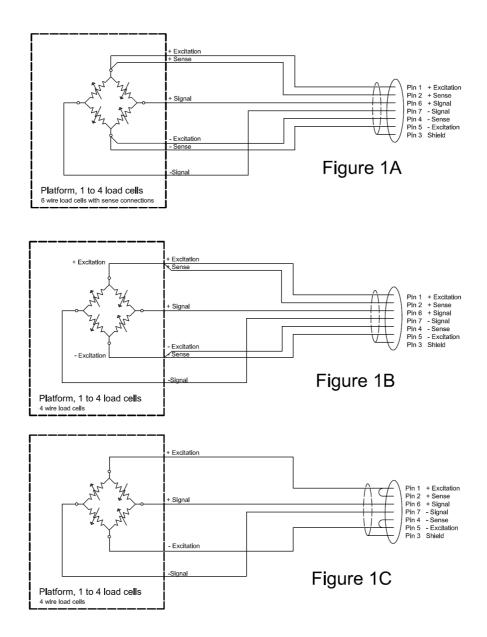
GK-M model must use the 6 wire connection and has certain limitations for wire size and length. Refer to the Approval Test Certificate for details.
