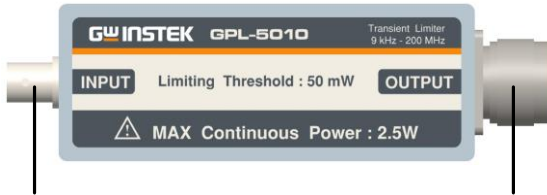
Input Interface: BNC female
