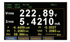
Irms is less than or equal to 60% of the previous setting range, so range is shifted down to 10mA.
