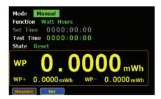
Press Enter button to enter Mode item. Use up and down arrow keys to toggle between Manual and Standard mode. Press Enter button again to confirm your selection.
