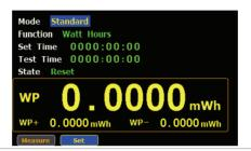
6. Press down arrow key to select **Function** item in the integrator measurement setting screen.
