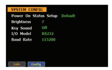
4. Press **Enter** button to enter **SYSTEM CONFIG** setting screen.
