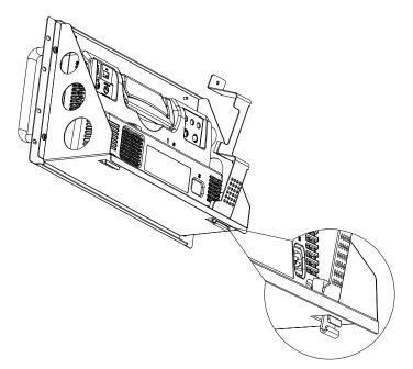
Test Equipment Depot - 800.517.8431 - 99 Washington Street Melrose, MA 02176 TestEquipmentDepot.com 3. Screw the left and right fasteners to the rack with the embossed nuts(6010-L00040S1).
