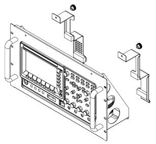
2. Insert the left and right fasteners into the two holes in the bottom cover.
