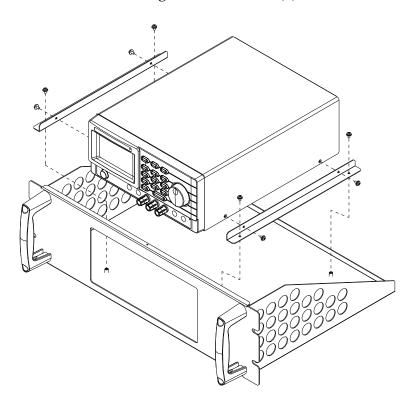
3. Place the PSP-405, PSP-603 or PSP-2010 units in the Bottom Chassis(4) and attach both Brackets(5) to the Bottom Chassis(4) using the BMS-W-3\*6(6) screws.
