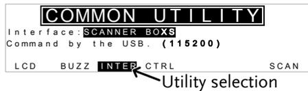
The Common Utility menu is accessed by pressing the UTILITY key when the tester is in VIEW status.
