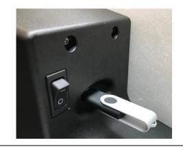
4 Press and hold **Menu** and ← buttons simultaneously while switching the power button ON for 3 seconds.
