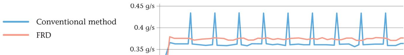
Flow rate measurement using FRD as opposed to the conventional method
