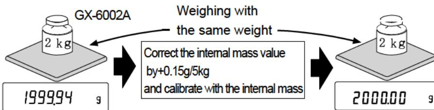
After performing one touch calibration, place the external weight on the balance and check the correction amount.
