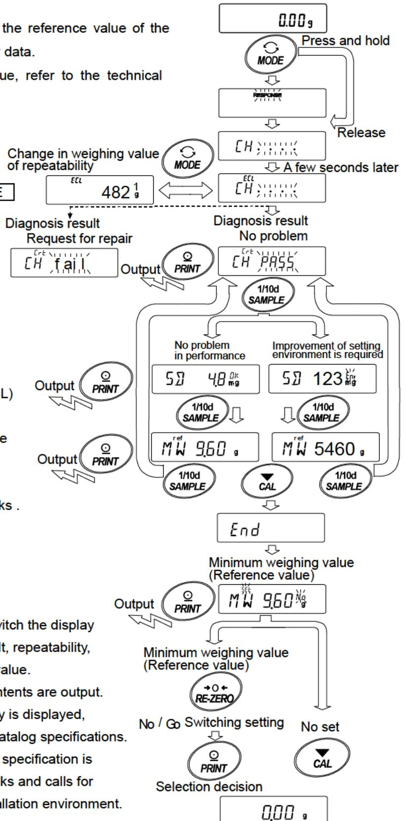
5. Press the **CAL** key to display **End** and move to the display for minimum weighing value registration.
