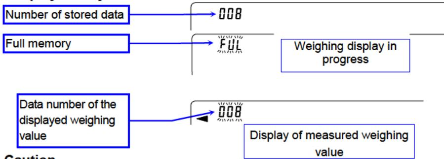
When the volume of measured values stored reaches its maximum, **ful** ← **dat** blink in turn.
