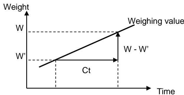
For flow rate calculation time Ct, select manual / automatic and set.
