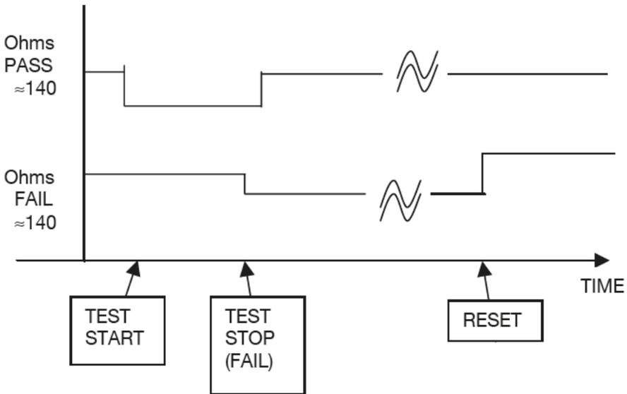
The **'Mode Contacts'** socket may be connected to a remote push-button switch or **no-volt** contact for resetting any fault status on the Hal, by activating the button or contact once only. Any further activation in this mode will default the Hal to its main menu. This is the same for the GREEN button which can be operated externally, in this way.
