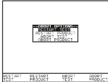
Use the function keys or the encoder to highlight an action following abort and press the green button to select the desired option.
