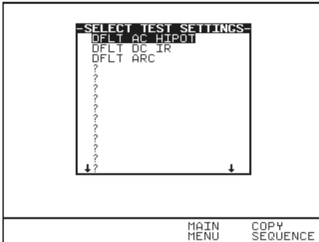
Use the encoder to highlight a Test Setting and press Green to enter the Test Settings Editor: -
