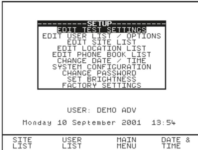
From this menu you can change the way the Tester will operate and also change user levels and sites. Use the encoder to highlight a function and press Green to select the desired option.
