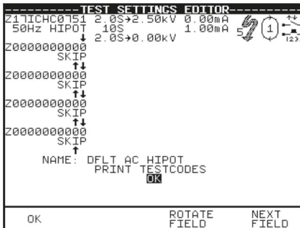
Use the encoder to highlight a field to be changed and press Green to select the desired option. Use the fast key to highlight the desired field, and the encoder to cycle through the range of permissible values for the test parameter. Use the fast key to enter the value. To exit this editing phase, select the OK fast key. Changes will be stored to the system. These fields have been described in detail under the Default Test Settings section.
