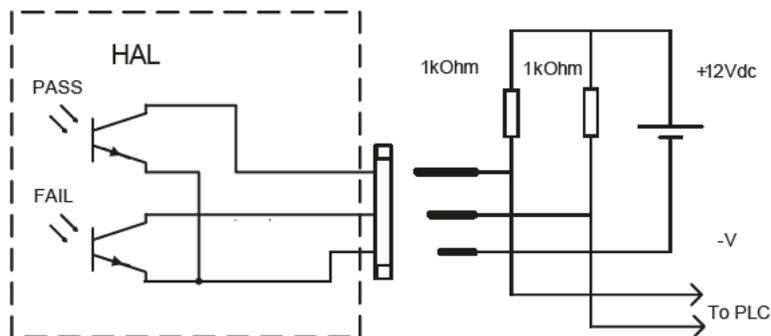
The Pass and Fail outputs follow the behaviour of the Indicators on the front of the tester, and are shown below. PLEASE NOTE THAT THE DIAGRAMS SHOW THE TYPICAL ON RESISTANCE FOR THE OPTOCOUPLER DEVICES WITHIN THE HAL.
