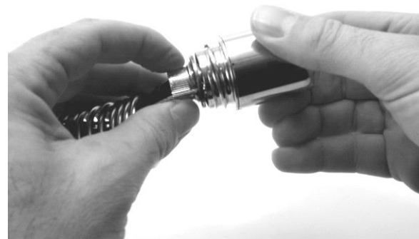
Figure 4 – Remove the Camera Head from the Locking Sleeve. DO NOT TWIST THE CAMERA! TWIST ONLY THE LOCKING SLEEVE!
