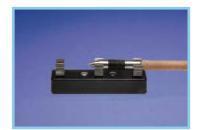
Moisture content standard used to verify moisture meter calibration. Has electrical resistance values of 16% and 22% to test against.
