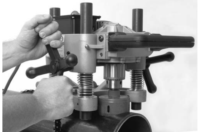
Figure 11 – Operating the Hole Cutting Tool
