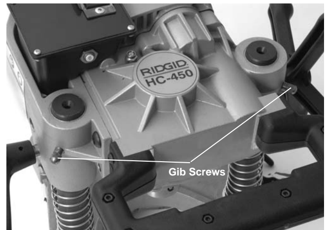
Figure 13 – Adjusting Gib Screws
