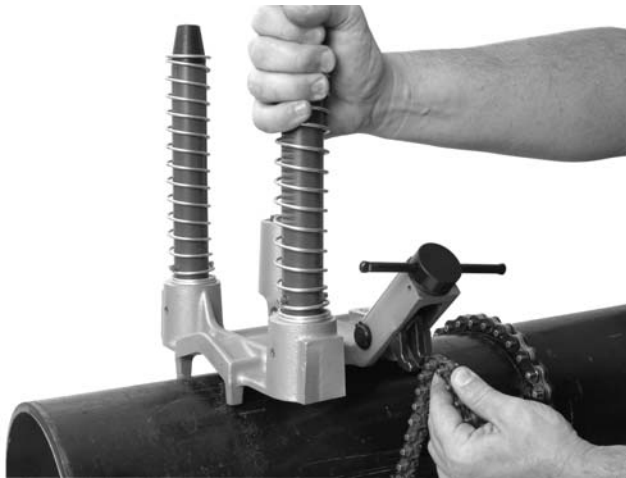
Figure 8 – Hooking the Chain
