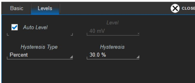
The default **Auto Level** selection will analyze the input signal to determine the logic high and low levels that produce the best Differential Manchester decoding. For most applications, this will be sufficient, and we recommend leaving it selected.
