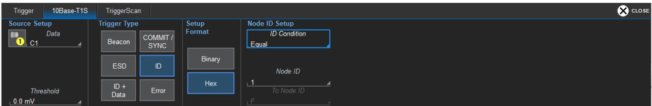
ID is used to trigger on the next packet from either a specific node ID or any value relative to a reference ID (e.g., greater than x).
