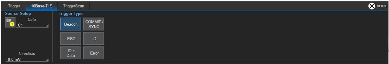
Select **Beacon** to trigger on the next packet sent from the Beacon (node ID0).
