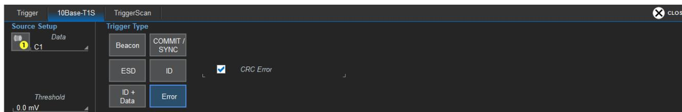
Choose **Error** to trigger on the next protocol error detected. Check **CRC error** to include | limit the trigger to Cyclic Redundancy Check errors.
