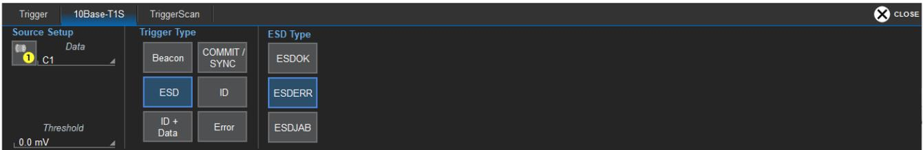
Select ESD to trigger on any of three End of Stream Delimiter conditions:
