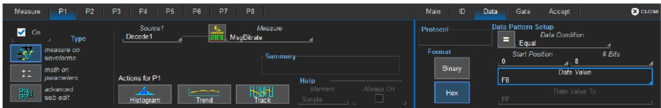
Use the same procedure as above to create a condition describing the **Data Value(s)** to include in the measurement. Use "X" as a wild card ("Don't Care") in any position where the value doesn't matter.
