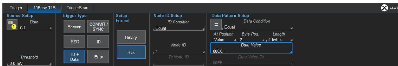
In addition to defining the node ID fields (above), create a condition statement that describes the Data field pattern upon which to trigger. This condition is added to the ID condition.
