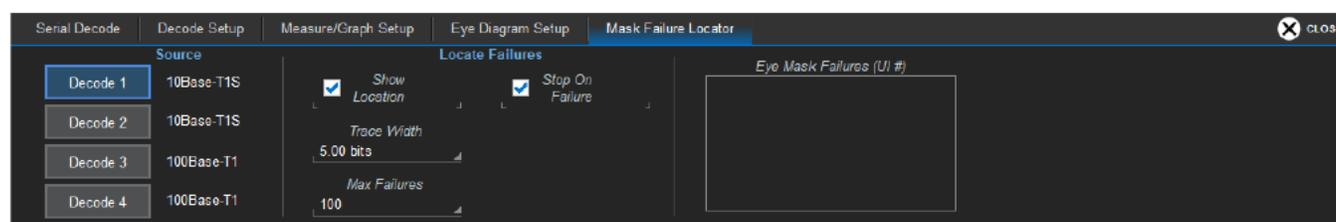
Check **Failure Location** to mark the failure on the source trace. Check **Stop On Failure** to stop acquisition whenever an eye mask failure occurs.
