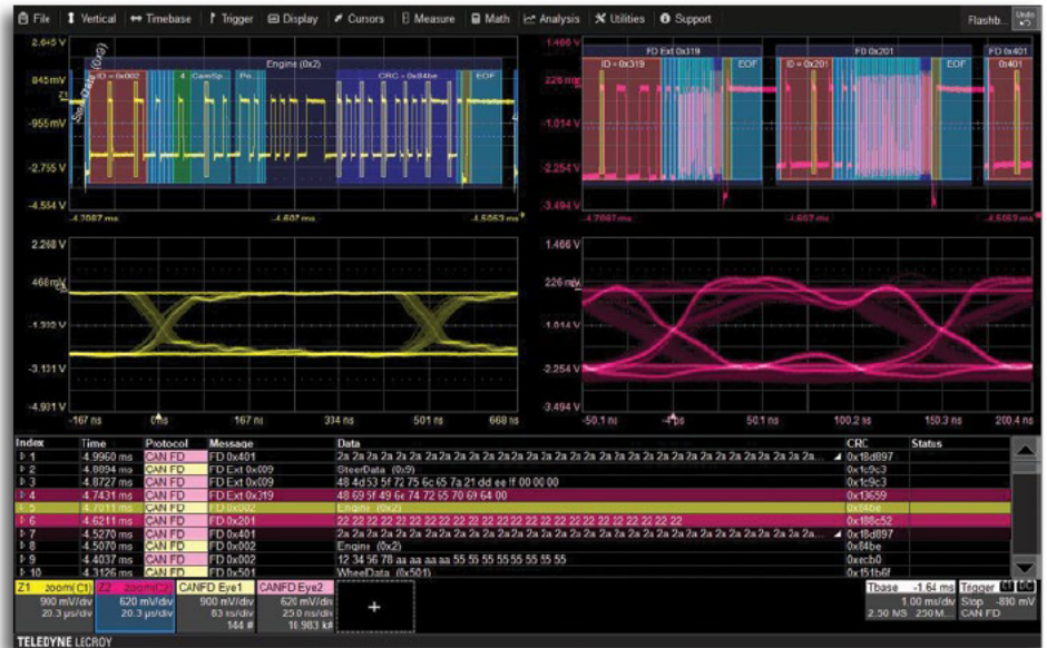
Eye diagrams “slice” each bit and overlay them to get a consolidated view of signal quality. Intrusions into the eye opening or onto a mask indicate potential problems.
