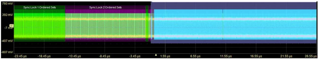
Initial decoding of USB4 waveform. At this resolution, very little information is visible on the overlay.
