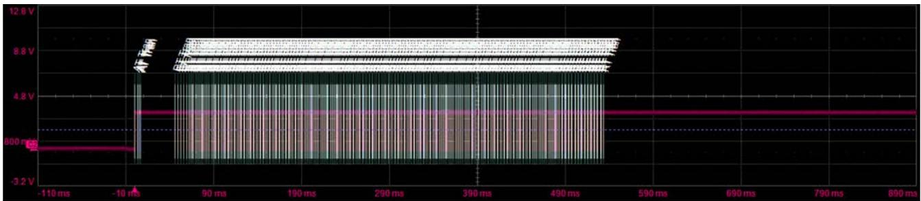
Initial decoding of USB4 sideband waveform. At this resolution, very little information is visible on the overlay.
