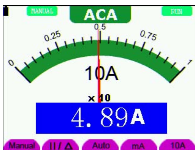
figure 30: AC Current Measurement for 10A
