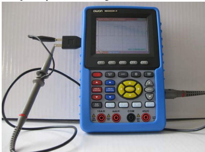
Fig.3. The connection of Square-wave test signal
