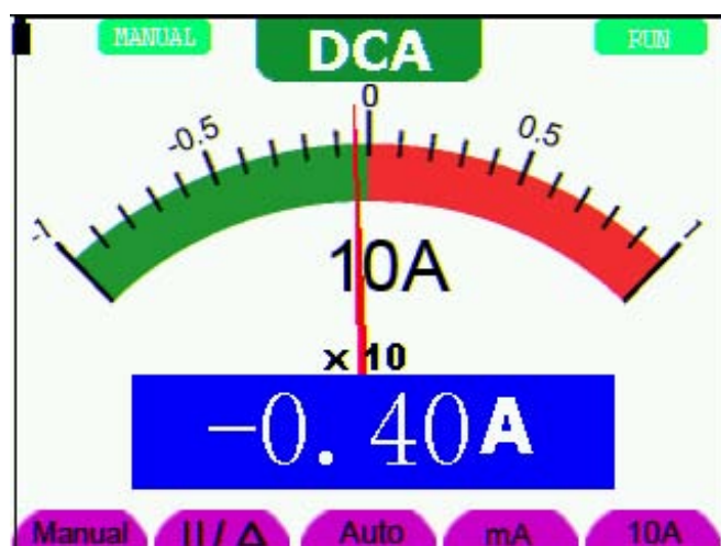
figure 28: DC Current Measurement for 10A
