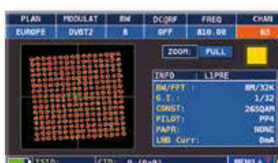
DVB-T2 (opt.) rotated Constellation 256 QAM mod., on the right relative modulation parameters & M-PLP
