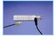
Uses the same contact pins that are mounted on each meter, providing 5/16" penetration. Used on wood up to an inch thick and drywall.
