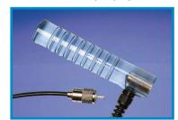
Electrode handle that attaches to the top of the meter. Used with 830-5 prod for baled hops.
