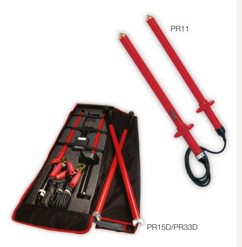
The PR11 provides a means of phase comparison at the point of paralleling two circuits, without the interposition of voltage transformers or secondary wiring earthed neutral systems. A neon type instrument, it is designed for use on earthed neutral systems up to 11KV. The PR15D / PR33D units enable phase angle comparison on earthed neutral systems up to 15KV and 33KV respectively.
