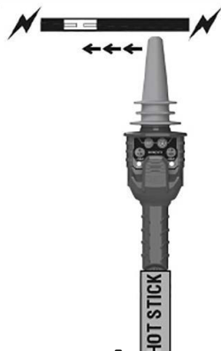
Fig. 2: Finding a cable fault
