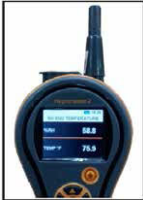
Figure 4: Hygromaster2 as a Hygrometer
