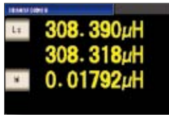
Transformer measurement mode Mutual inductance measurement screen
