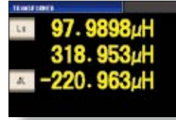
Transformer measurement mode Inductance difference measurement screen
