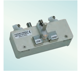
SMD TEST FIXTURE 9699 Electrodes on bottom for SMD DC to 120 MHz Test sample dimensions: 1.0mm (0.04in) to 4.0mm (0.16in) wide, maximum 1.5mm (0.06in) high
