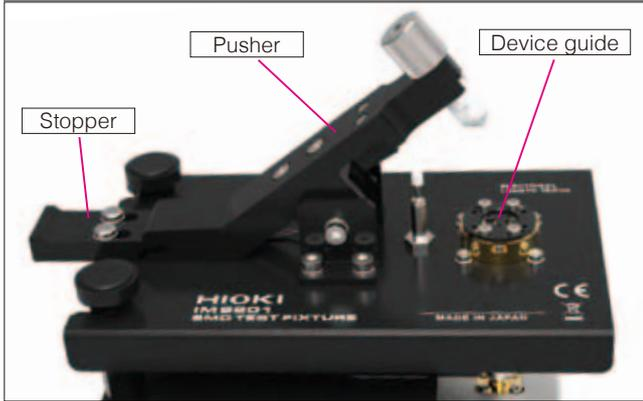
2. Release the stopper and anchor the pusher to secure the component
