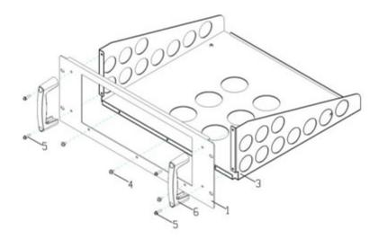
4. Place the unit on top of the holding bracket followed by fastening them with 2 screws 594B-W4008NS1.
