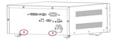
2. Fasten the 2 screws, which were removed from the step 1, with the holder 62RA-445HP101 on the rear side of unit.
