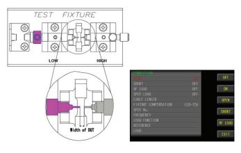
4. Pull the LOW side test pin leftward and loosen the High side locking screw followed by moving the HIGH side test pin leftward to the center of test stage and fastening the locking screw. Loosen the LOW side test pin to have the test pins of both LOW and HIGH sides contacted in short circuit. Implement short circuit test to make SHORT item displayed ON.
