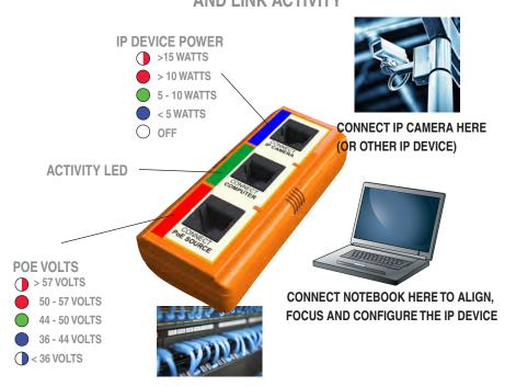
CONNECT POE POWER SOURCE HERE (POE SWITCH OR INJECTOR)
