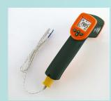
Compact non-contact InfraRed (IR) Thermometer measures up to 1112°F (600°C) with built-in laser pointer to identify target area and improve aim. Type K input allows for high temperature measurements up to 1832°F (1000°C). Builtin temperature sensor also measures Air Temperature. Adjustable emissivity feature allows for a higher accuracy when measuring temperature on various surfaces.
