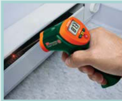
Test for temperature in heating systems
