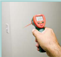
Check building for insufficient insulation
