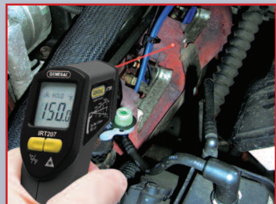
With a 600°F measurement ceiling, the unit can handle any automotive application
