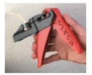
Ensure jack is completely and securely inserted in jack holder bed with IDC slots facing the blades.
