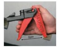
3. Make sure handle is open. Once pin #1 has been inserted, slide pin #2 into blade head.
