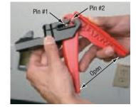
2. Angle handle, and insert pin one into blade head first. Be sure to keep tool handle in open position.
