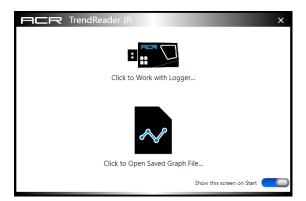
You can choose to access and work with the JR2000 data logger, by clicking the top icon, or accessing saved graph files by clicking the lower icon.
