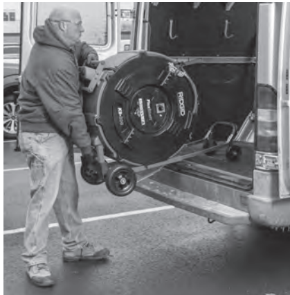
Figure 14 – Lifting Unit Onto Vehicle
