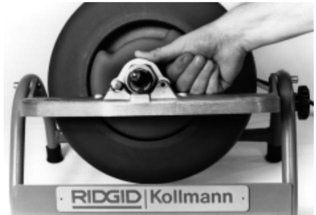
**Figure 3 – Locking Front Bracket**
