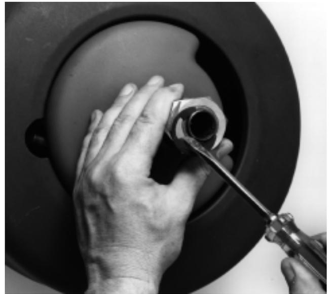
**Figure 14 – Removing E-Clips**
