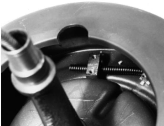
**Figure 16 – Position New Cable Under Bracket**
