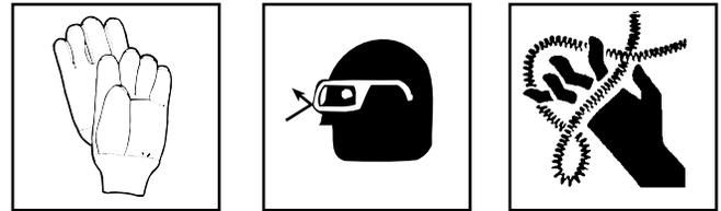
Wear gloves provided with machine. Never grasp a rotating cable with a rag or loose fitting cloth glove that may become wrapped around the cable, causing serious injury.
