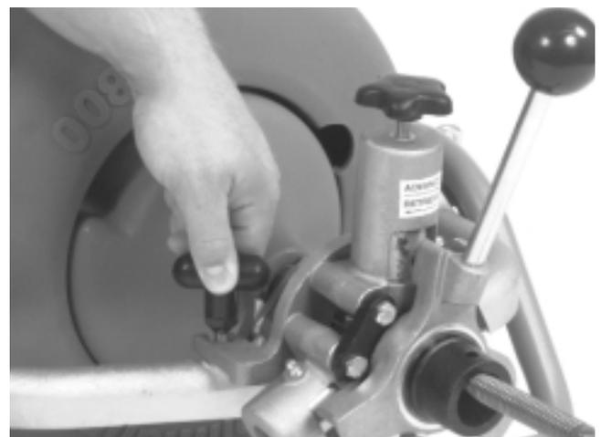
**Figure 4 – Mounting the Autofeed Onto the Frame**
