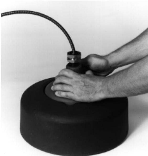
**Figure 13 – Removing Cable End**
