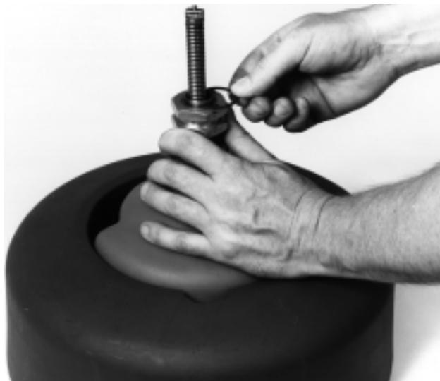
**Figure 17 – Reassemble Inner Drum, Front Bracket and E-Clips**
