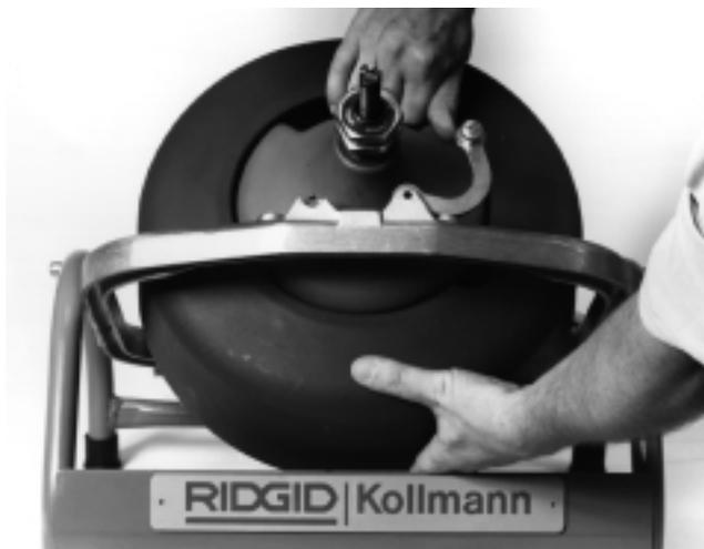
**Figure 2 – Aligning Drum and Gearbox Bore**
