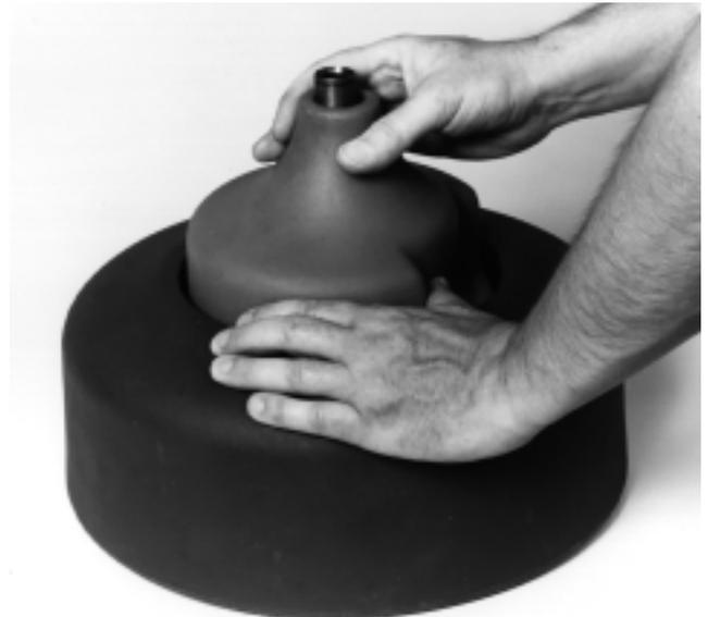
**Figure 15 – Removing Inner Drum**
