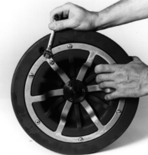
**Figure 12 – Loosen Cable Bracket**
