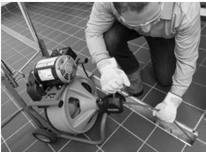
Figure 15 – Operating K-400 with AUTOFEED
