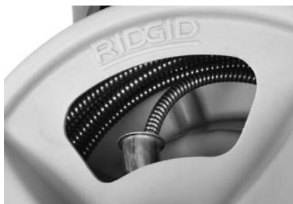
Figure 18 – Coil Cable Into Drum As Shown
