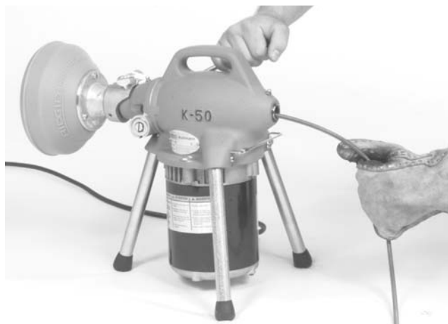
Figure 5 – Cable Adapter Attachment
