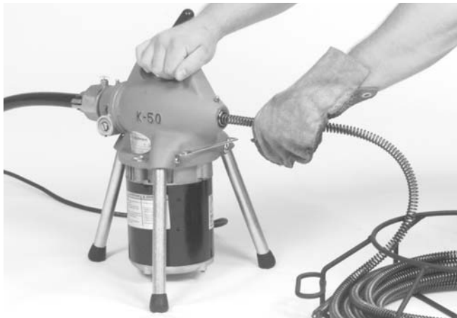
Figure 3 – Inserting Cable Into Front Of Machine
