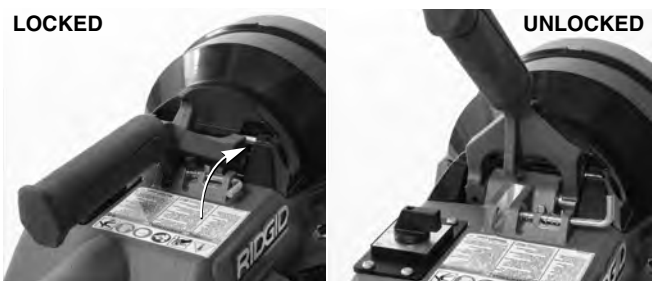
Figure 4 – Releasing the Clutch Handle
