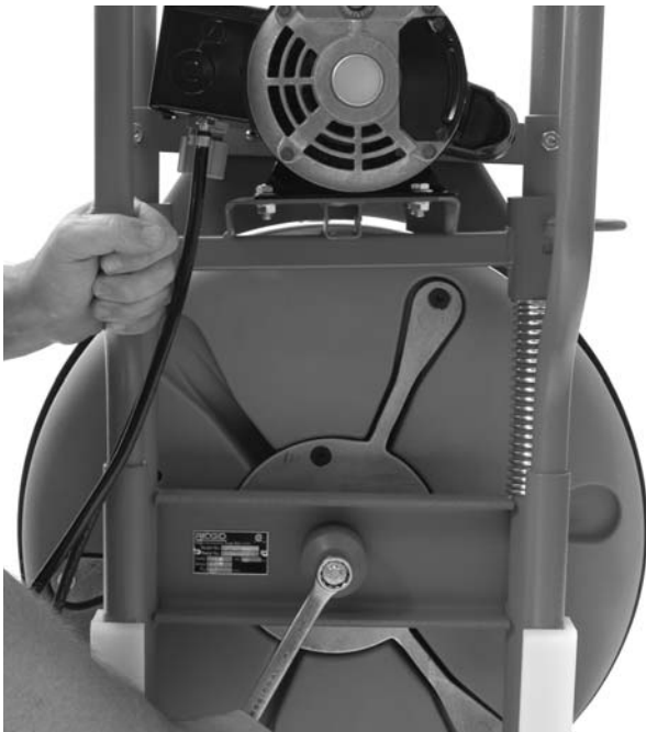
Figure 18 – Removing Drum Bolt
