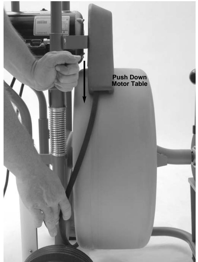
Figure 17 – Releasing Belt Tension
