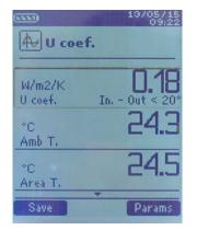
The device displays the U coefficient, the surface temperature, the ambient temperature and the external temperature.
