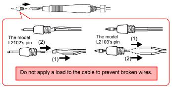
5. Fasten a new pin. Press the tip of the pin against a desk so that the pin won't spring out, and push the connector onto the pin
