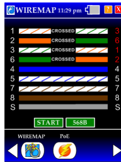
Example - Crossed 12-36 shielded cable
