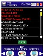
Top talkers displays the MAC address, IP address, Device Name, the number and percentage of transmitting frames on the network in order from the highest used bandwidth to the lowest.
