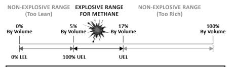
BELOW a specific LEL for a combustible gas, the mixture is too "lean" (not enough gas is present to burn). See the above visual diagram that applies to Methane only.
