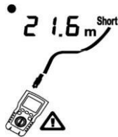
Figure 6.16 Short on Coaxial Cabling
