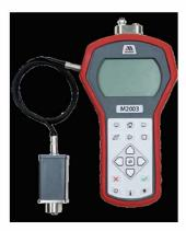
But that's not all. In Pressure mode, the M2003 displays pressure in a variety of Customary and SI measurements units. Selecting the ALT or IAS switches the M2003 to Altitude mode for us in checking altimeter instrumentation. Customary or SI measurement units for Altitude and Indicated Air Speed are selectable by the customer.
