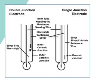
This junction can become clogged by particulates in the solution and can also facilitate poisoning by metal ions present in the solution. If a clogged junction is suspected it is best to soak the electrode in tap water to dissolve the material and clear the junction. When not in use it is best to store the electrode in either buffer 4.0 or buffer 7.0. Never store an electrode in distilled or deionized water as this will cause migration of the electrolyte solution from the electrode.
