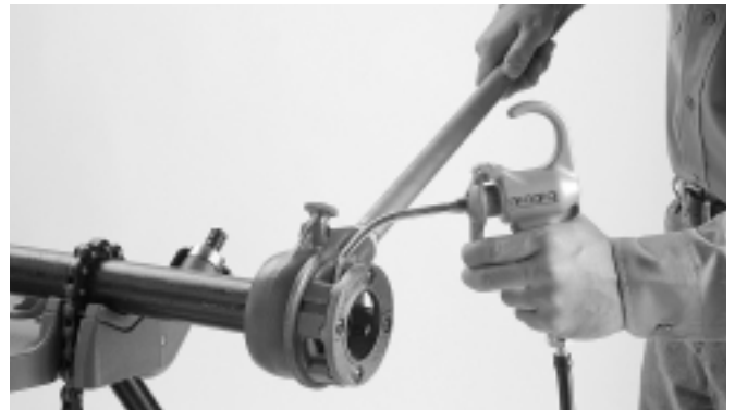
Figure 4 – Applying Thread Cutter Oil
