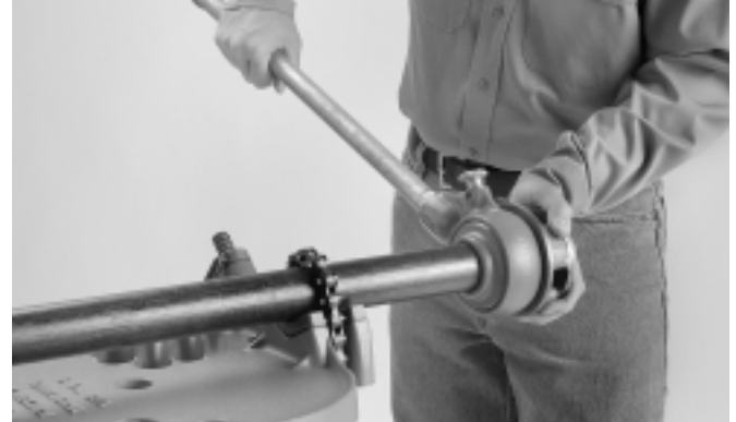
Figure 3 – Sliding Threader On Pipe
